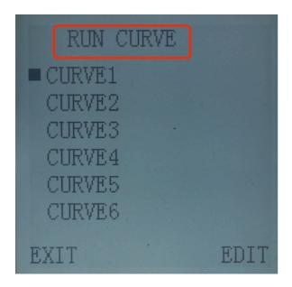
2) Press the arrow keys to select the CURVE that you want to run, press ENTER to enter the curve running interface
