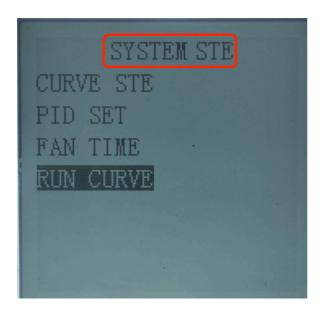
1) Press the arrow keys to select the RUN CURVE, press ENTER the RUN CURVE Interface.
