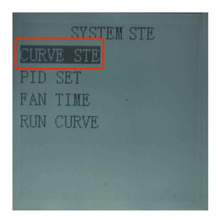
2) to enter the the curve selection screen, press the arrow keys to select the curve which you want to modify.
