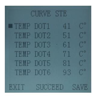
The basic definition of the curve, each curve can be set to 45 temperature point, the heater's temperature will be in accordance with the 45 target temperature. Each temperature point's interval is 10 seconds, so the curve's longest heating time is 450 seconds, the first 0 value point is the end of this curve.
