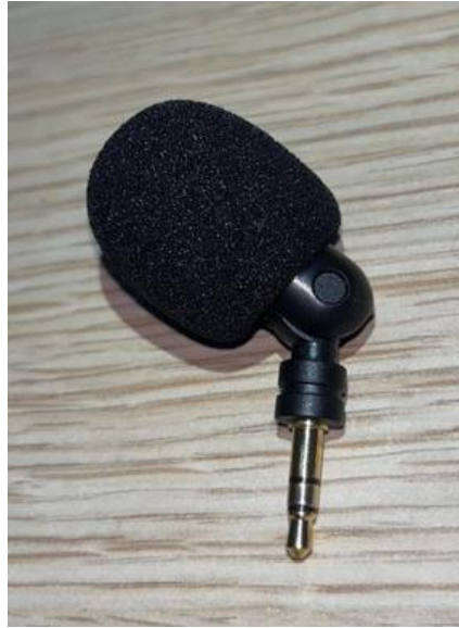
Figure 19: Primo EM272 microphone with windshield installed.
