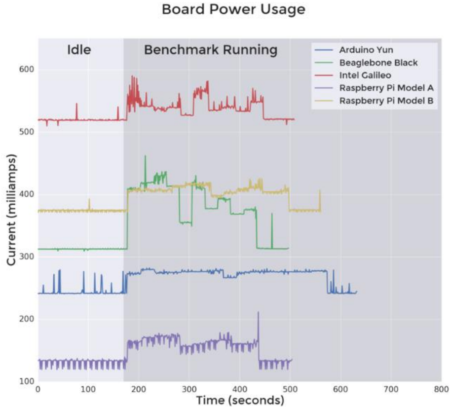
Figure 2: Comparative graph of current consumption (in mA) for different models of SBCs and Arduino.
