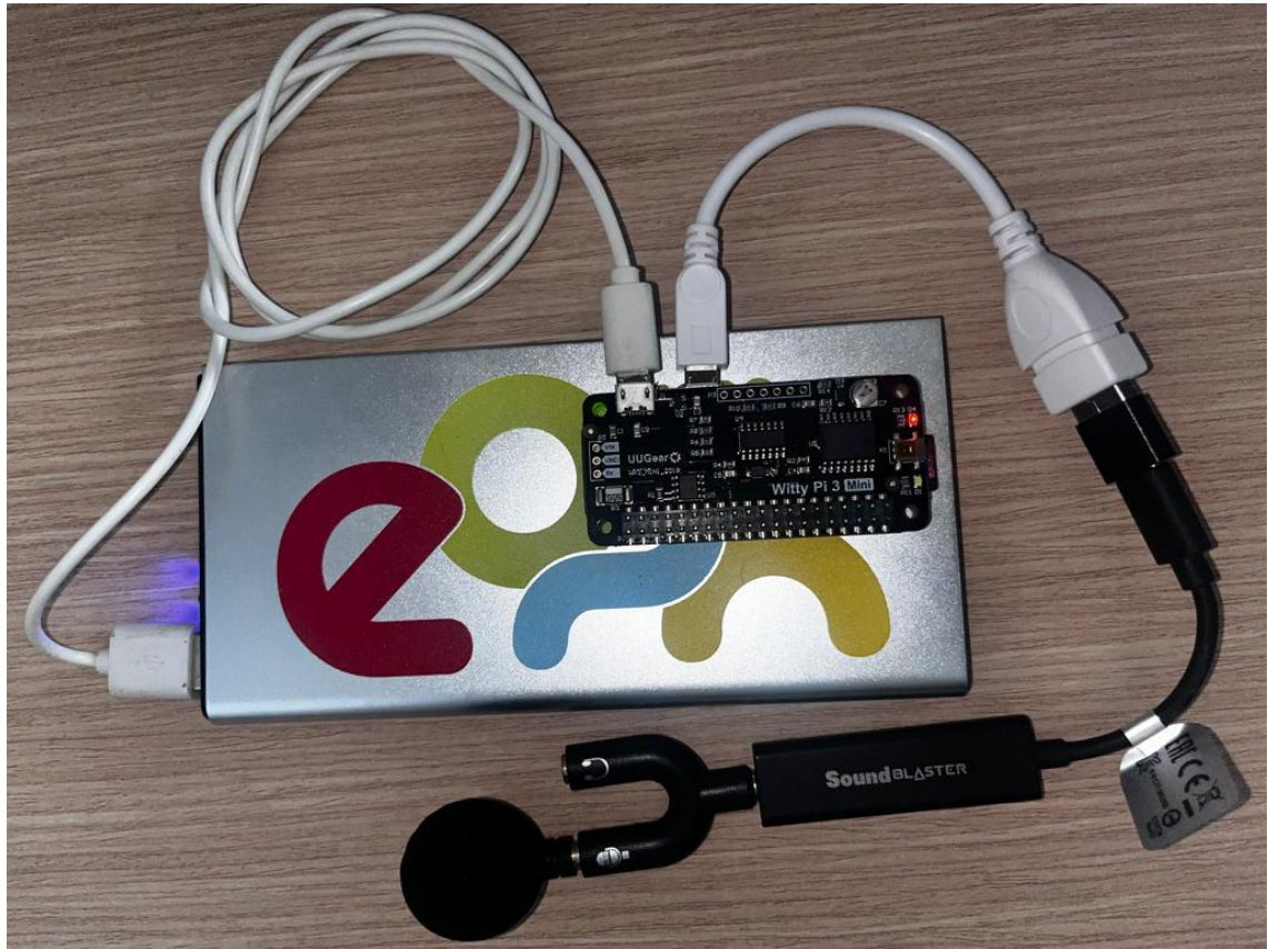
Figure 35: Image of the complete first version of the SOLMoth device without an external casing
